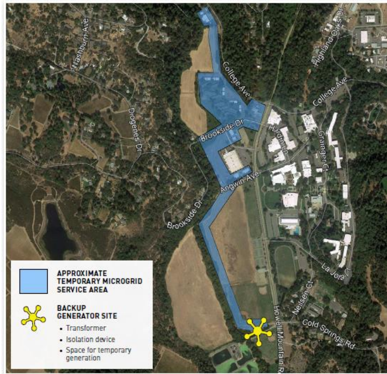
Figure 12: Approximate Energization Area of Angwin Temporary Microgrid
