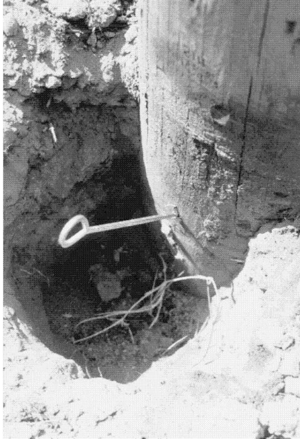
Figure 5. Using a Shell Thickness Gauge
