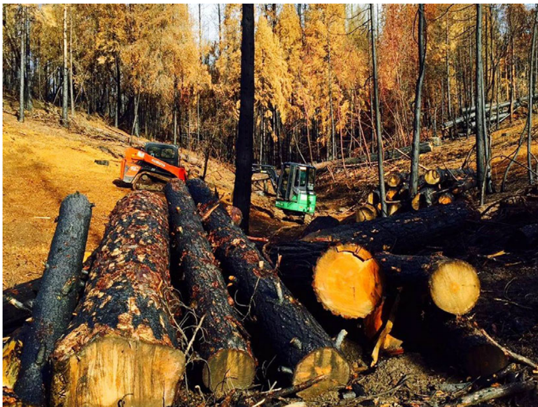
Photo 24- AVOID THIS! Avoid using equipment in draw bottom. Avoid operating equipment within WPZ (25 feet of this ephemeral draw). Do not pile debris or logs in draw.
