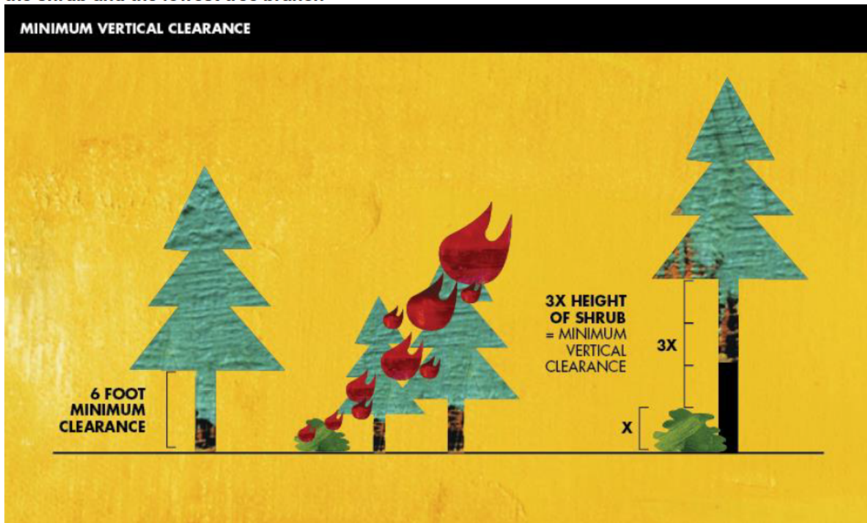
Figure 3. A Five Foot Shrub is Growing Near a Tree. 3 \times 5 = 15 feet of clearance needed between the top the shrub and the lowest tree branch
