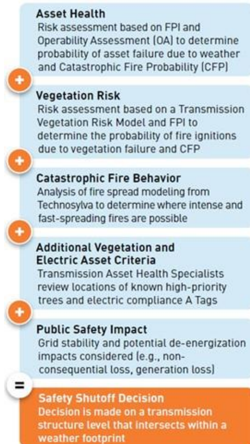
FIGURE PG&E-9.2.1-6: VISUAL REPRESENTATION OF TRANSMISSION SCOPING
