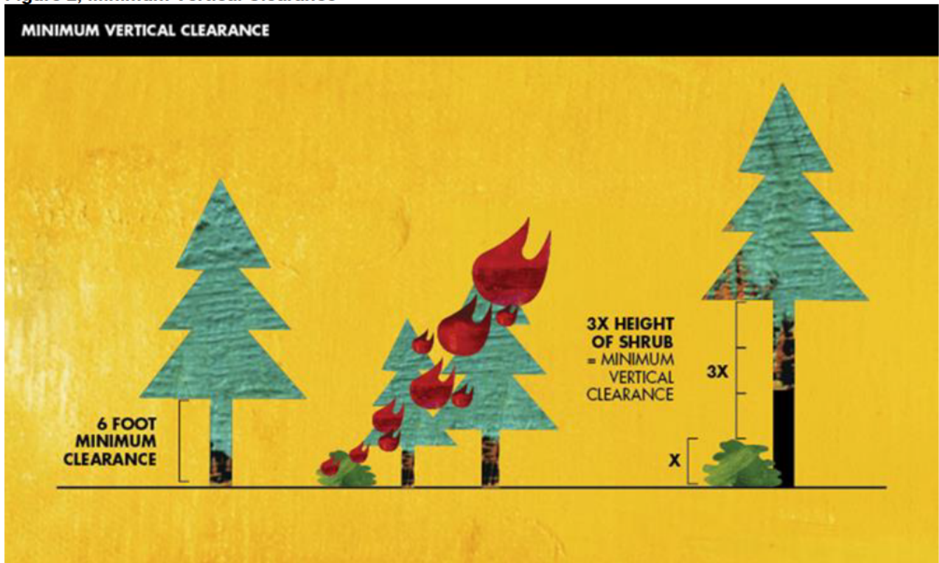
Figure 2, Minimum Vertical Clearance
