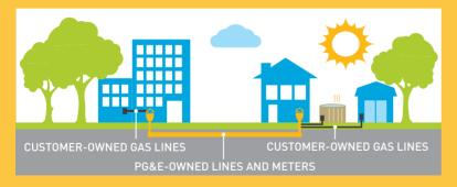
PG&E is responsible for maintaining the system that delivers natural gas, up to and including the gas meter. Customers are responsible for the maintenance of customer-owned piping on their property.
