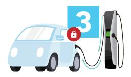
During charging, the cable is locked to the car.
