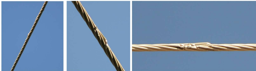
Conductor slap damage (molten droplets, broken strands)
