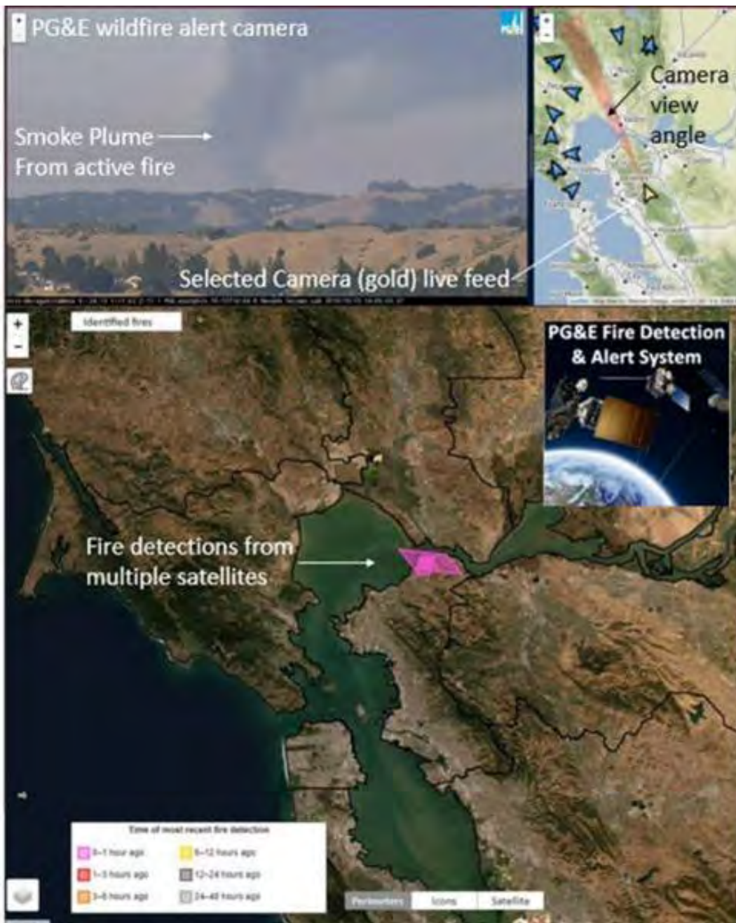
FIGURE PG&E-7.3.2-12: EXAMPLE INTEGRATION OF PG&E WILDFIRE CAMERAS AND THE PG&E FDAS –THIS EXAMPLE SHOWS A SMOKE PLUME VISIBLE FROM A FIRE DETECTED FROM FDAS – THIS EXAMPLE IS FROM THE FIRE THAT OCCURRED IN THE NUSTAR ENERGY FACILITY IN CROCKETT, CALIFORNIA
