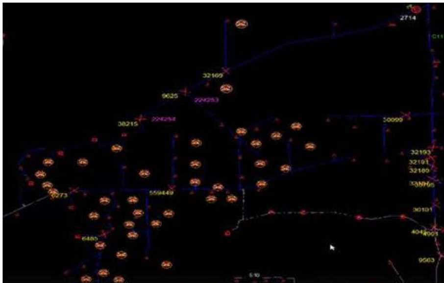
Figure 8. Example of Partial Voltage Outage Calls
