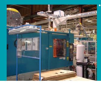
Plastic components manufacturers rely on injection molding machines to shape plastic products. Converting from constant volume hydraulic injection molding machines to variable volume machines can save energy because variable volume molding machines are more responsive to change in the molding process's demand patterns.
