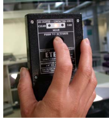
Figure 3: Meter shows LowE coating on the near side of glass.
