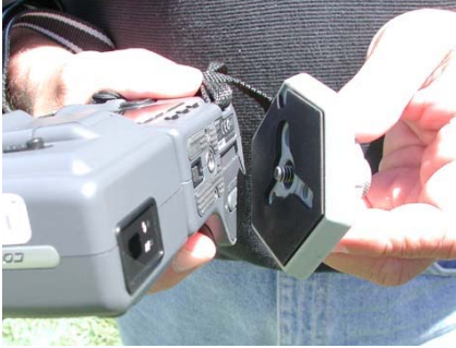
Figure 3: Attach mounting plate to base
