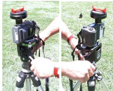
Figure 6: Leveling the camera parallel and perpendicular to camera body
