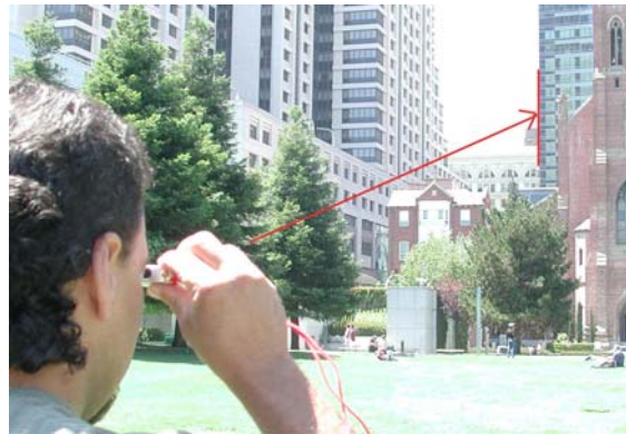
Figure 3: Aligning compass sight and distant object.
