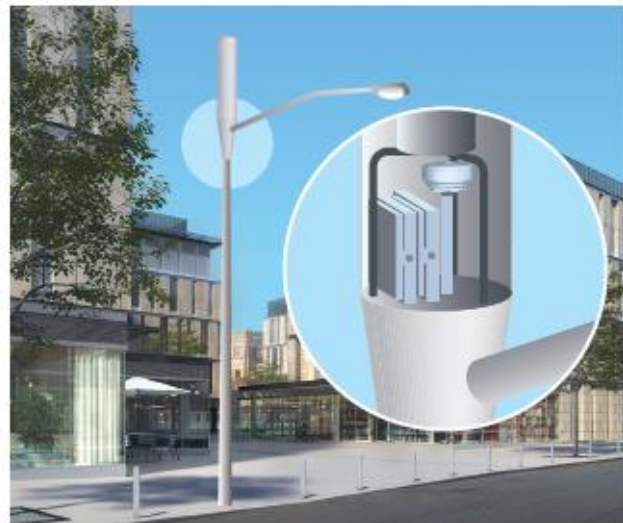
Existing pole - Retrofit - SmartMeter inside
