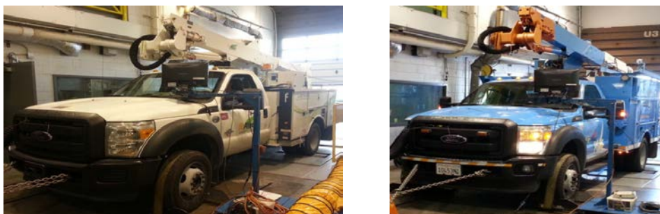
Figure 4-5 National Renewable Energy Laboratory (NREL) Refuel Lab Chassis Dyno Baseline Truck (left); PHEV Driveline Up-Fit Vehicle (right)
