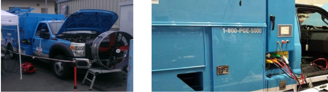
Figure 4-1 Mule Vehicles Under Test at ATS Including Auxiliary Vehicle Cooling
