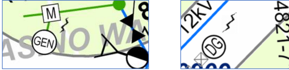
Figure 17: Primary and Secondary-connected Generators with Control Symbology (SCADA Lightning Bolt) in GIS
