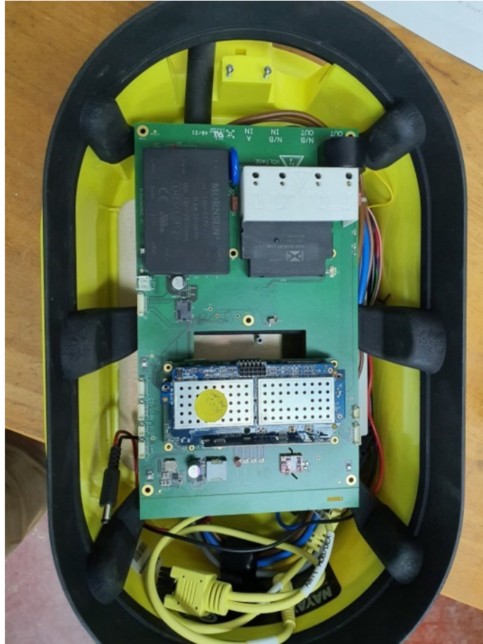
Figure 15. EVSE with NGM Core Installed
