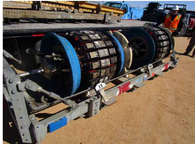
Figure 24 – ROSEN Electro Magnetic Acoustic Transducer (EMAT) Tool After an Inspection on L-300B
