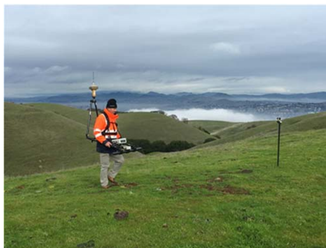
Figure 59 – Sample Project: Large Standoff Magnetometry (LSM)
