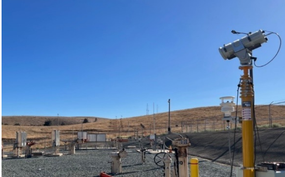
Figure 6: PG&E uses a QLM camera mounted on a yellow pole to continuously monitor and take measurements of intermittent devices at M&R station to accurately represent their emissions and establish an accurate emissions factor.
