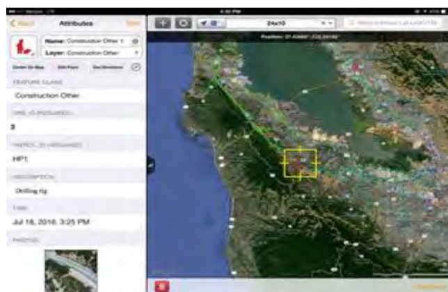
Figure 58 – Screenshot of iPad GIS Application Used by Aerial Patrol in Monitoring Potential Excavation Observations
