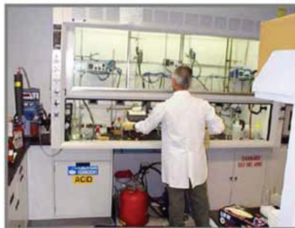
Figure 5.05 Hood with combination "A-style" sash.
