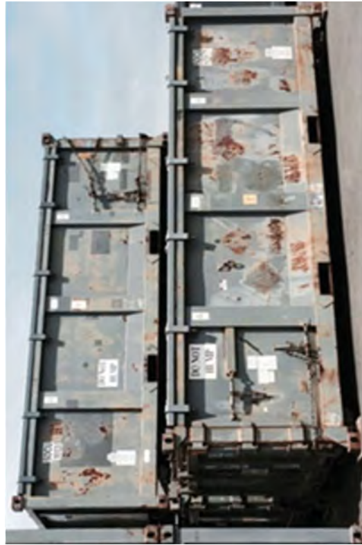
IP-2 containers that had to be refurbished and verified for integrity due to excessive rust.
