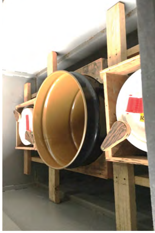
Using a secure hold down method for transporting drums in a B-25 box.
