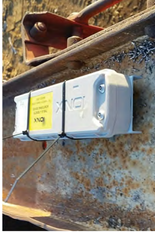
GPS units installed on every Railroad Gondola allowed them to be tracked by the waste group and rail company.
