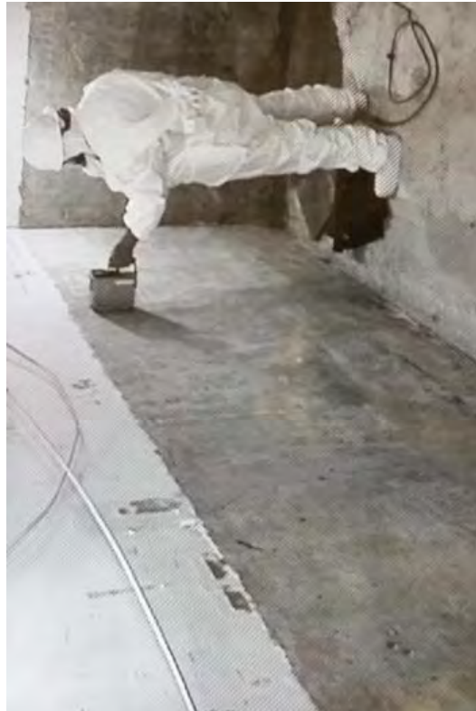
An RP technician surveying the concentrated waste tank room.
