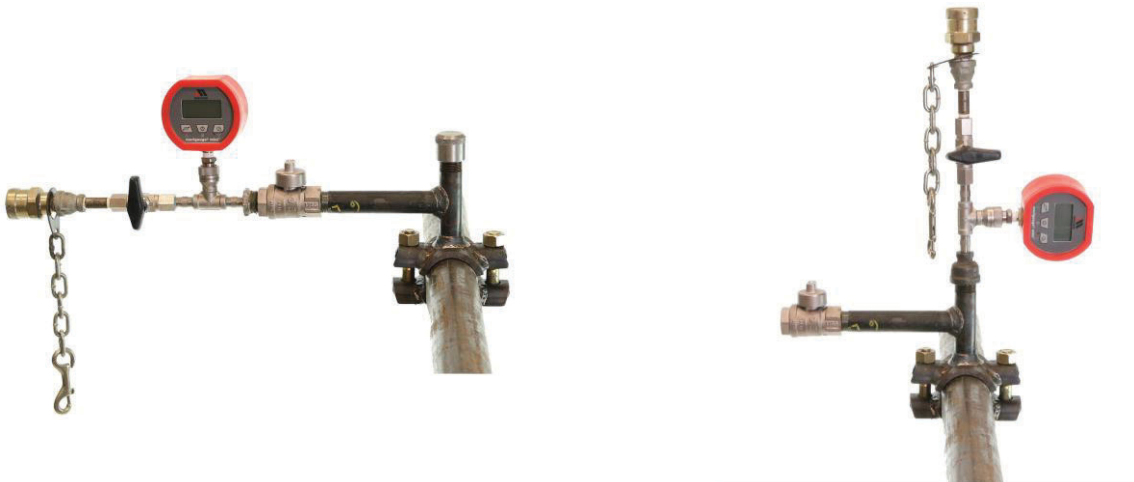
Figure 4. Typical Test Assembly Installed
