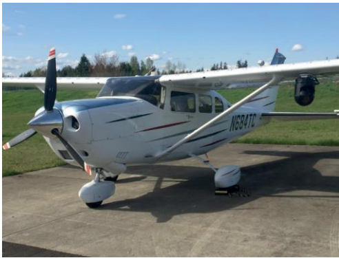
Figure 23 – Patrol Aircraft With Wing Mounted Camera
