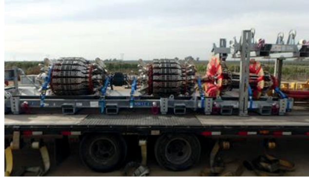
Figure 30 – ROSEN Electro Magnetic Acoustic Transducer (EMAT) Tool Before an Inspection on L-300A
