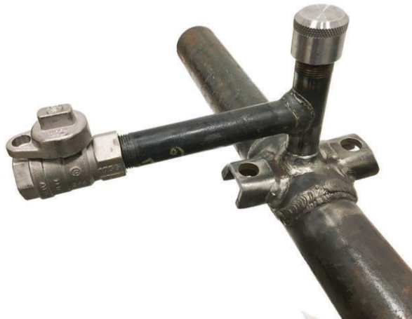
Figure 16. Complete Saddle Weld
