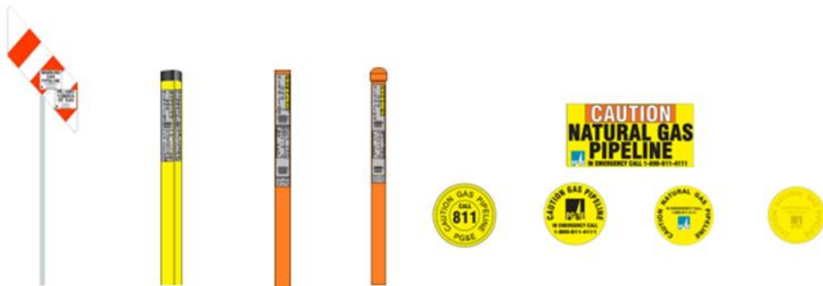
Figure 31 – Types of Pipeline Markers
