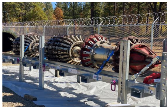
Figure 36 – Electro Magnetic Acoustic Transducer (EMAT) Tool After an Inspection on Line 400
