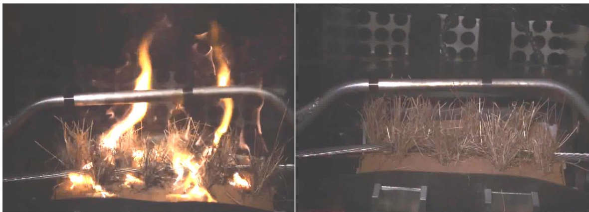
Figure 1 Victorian Ignition Testing of Energized Conductor - Without REFCL (Left), With REFCL (Right)
