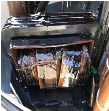
Figure 13 Failed internal PT inside voltage regulator
