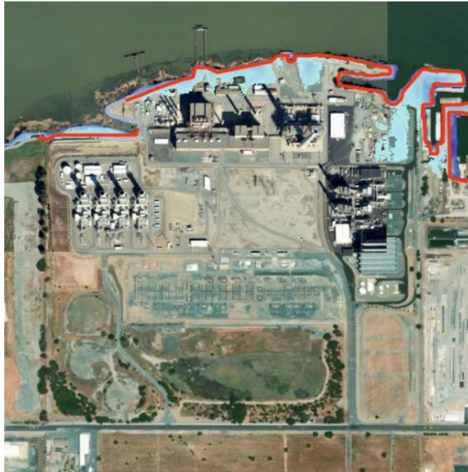
Figure 3.1.3-15. 2040 SLR inundation for a 100-year storm (Source: Bay Conservation and Development Commission)
