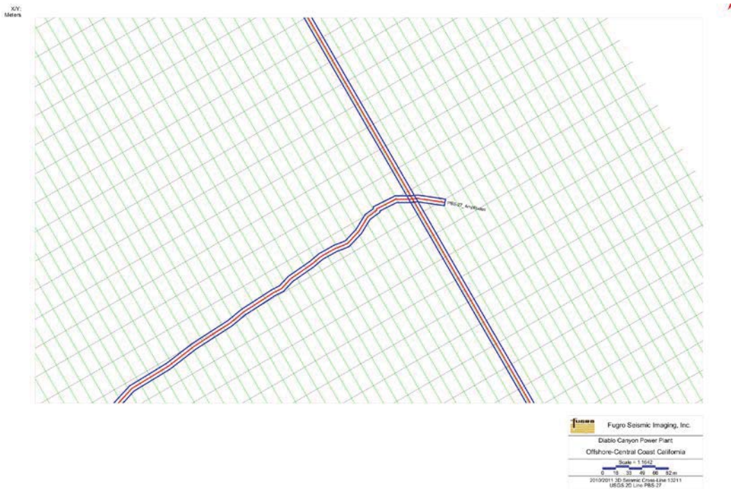
Figure 18. Intersections of 2010/2011 3D Seismic Survey Cross-Line 13211 and USGS 2D Line PBS-22. Several intersections were used to calculate time shifts needed to match the 3D Seismic Data set with the 2D Seismic data.
