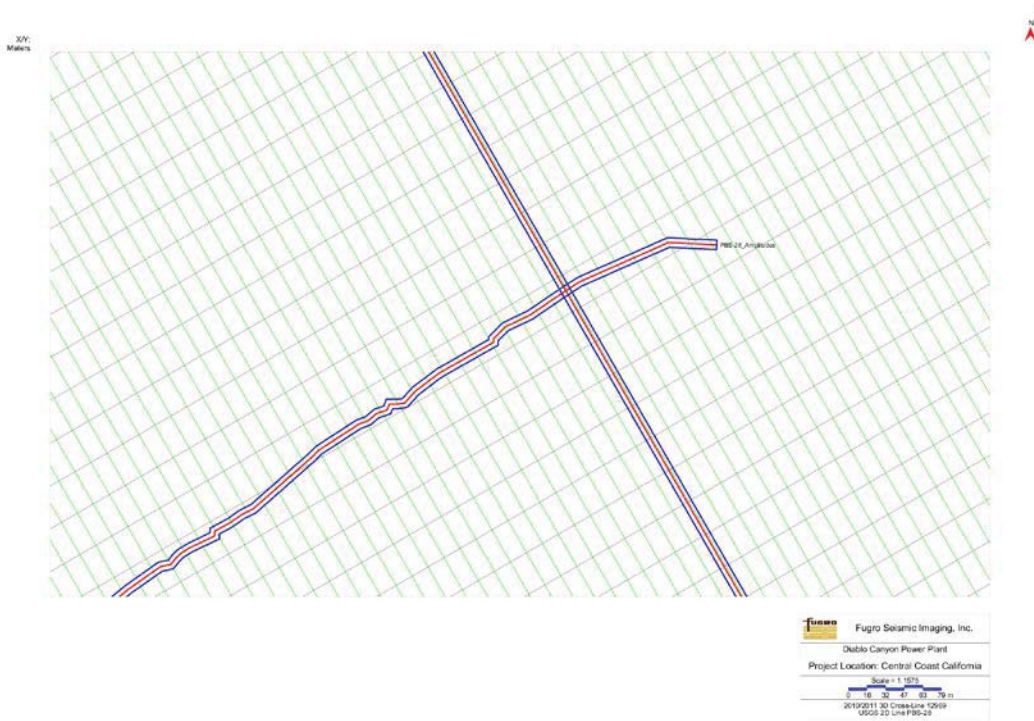
Figure 17. Intersection display of 3D Line 12969 and USGS 2D Line PBS-28. Time shifts were calculated in order to match the 3D dataset with the 2D data.
