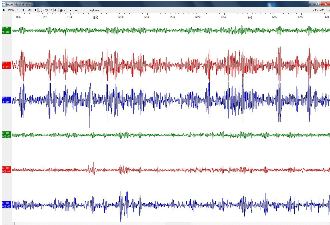
Fig. 13: The recordings of the three components of Temp-2 (upper three traces) and of Temp-1 (lower three traces) during the very two hour time window on 24 Sep 13, when the onsets of the Pakistan earthquake were expected.
