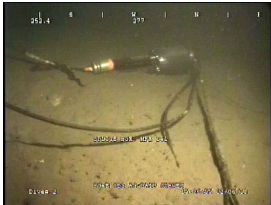
Figure 7. Video-Still of Junction Box Between OBS Units 4 and 3 (Water Depth 252 ft. [77m])
