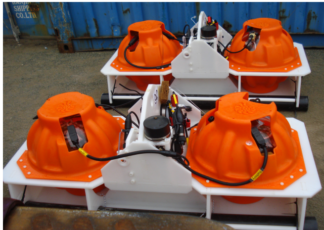
Fig. 1: The two instruments in their initial pre-deployment configuration. The glass spheres are covered with orange plastic protectors
