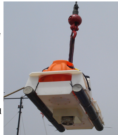
Fig. 2: Sensor mounted in center underneath the frame
