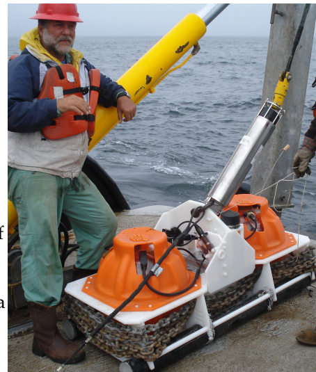
Fig. 3: One of the portable OBS shortly before deployment. Note the chains added to increase stability of the OBS.
