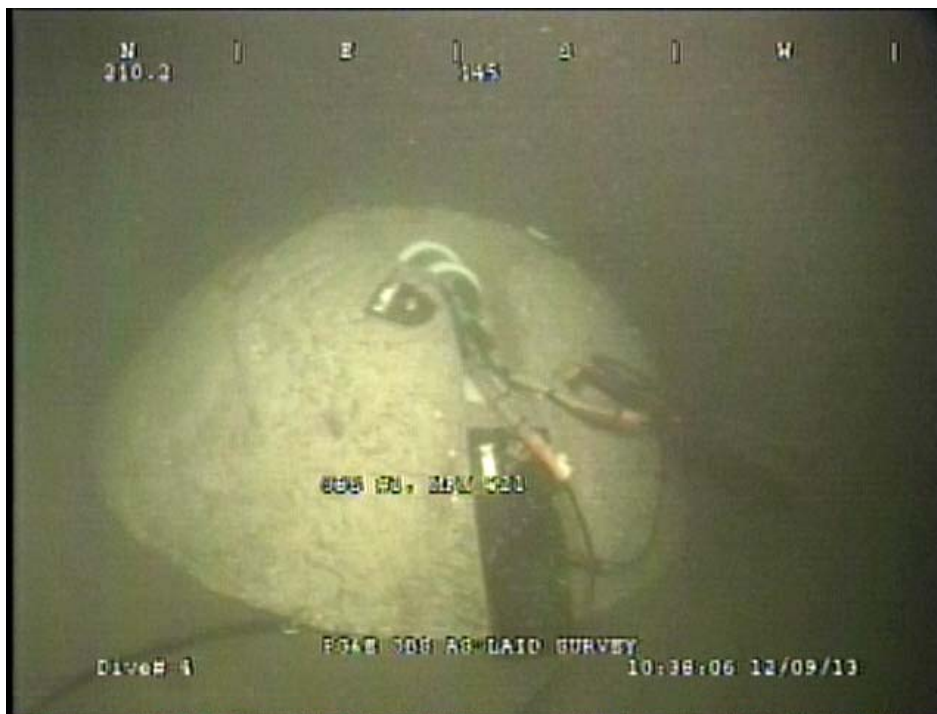
Figure 9. Video-Still of OBS-1 and Installation Bridle (Water Depth 210 ft. [64 m])
