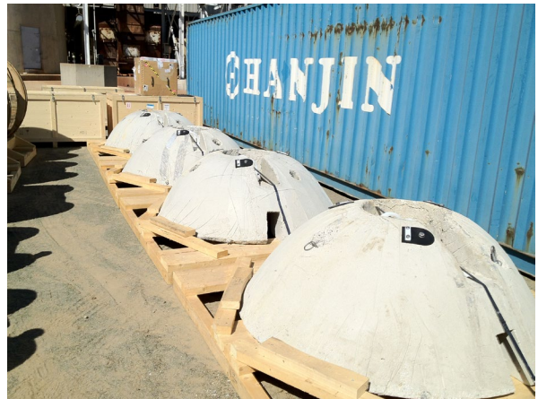
(d) Instruments protected by concrete caps (each measures 1 foot high and 6 feet across and weighs 1 ton)
