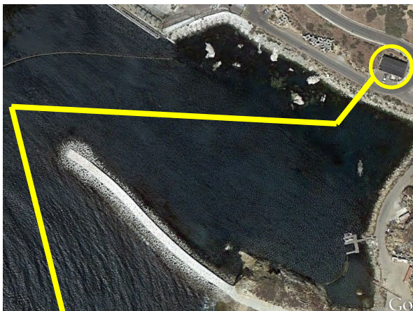
(c) Schematic of cable in DCPD intake (yellow line) to onshore recording center (yellow circle)
