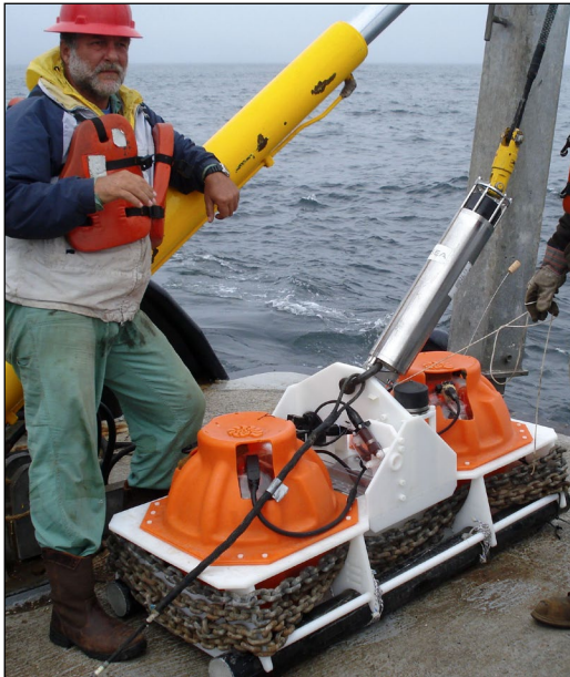
(c) One of the temporary OBS units shortly before deployment. Chains were added to increase the stability of the unit.
