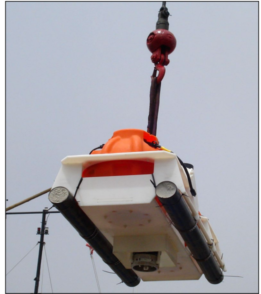
(b) Cement ballasts with the sensor mounted in the center underneath the frames.
