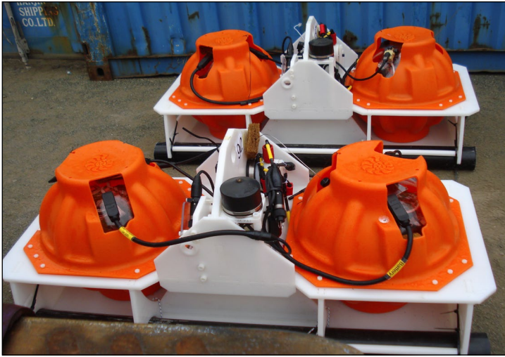
(a) Instruments in pre-deployment configuration. Instruments are covered with orange plastic protectors.
