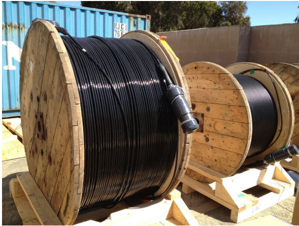
(a) Cable containing optical fiber for two-way data transmission and power from shore to the units
