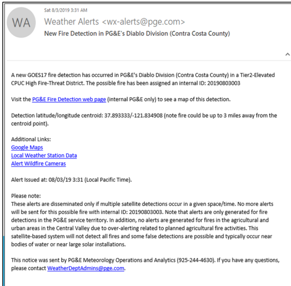
FIGURE PG&E 5-14: EXAMPLE FIRE DETECTION ALERT EMAIL DISTRIBUTED AUTOMATICALLY BY THE PG&E FIRE DETECTION AND ALERT SYSTEM – THIS INCIDENT WAS THE MARSH FIRE THAT WAS REPORTED IN CONTRA COSTA COUNTY ON AUGUST 3, 2019.
