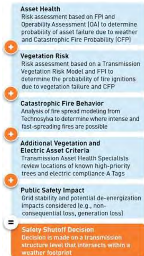
FIGURE PG&E-9.2.1-6: VISUAL REPRESENTATION OF TRANSMISSION SCOPING
