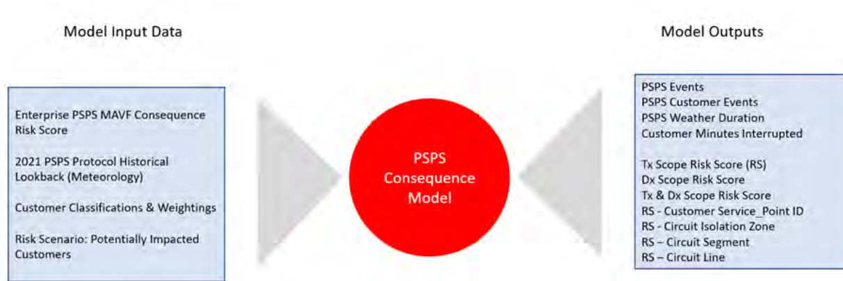
FIGURE PG&E-B-3: PSPS CONSEQUENCE MODEL BOW-TIE
