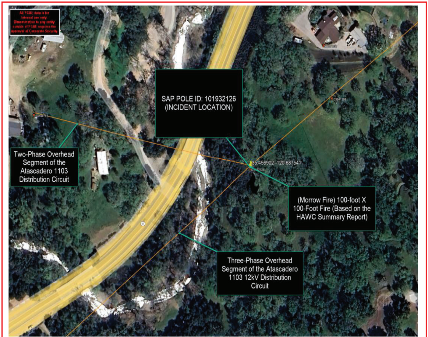
Figure 1 - Google Earth Diagram of the Atascadero 1103 12kV Circuit. The location of the fire is approximate based on reports and pictures provided.
