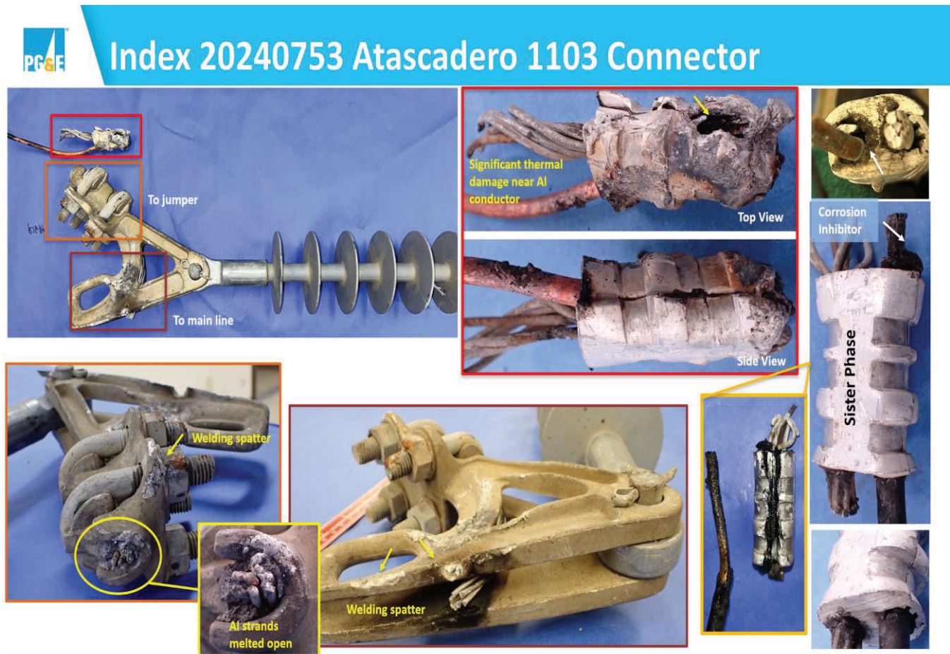
Figure 8 - An inspection of the collected materials revealed extensive thermal damage and material loss on the connector, particularly around the aluminum conductor.
