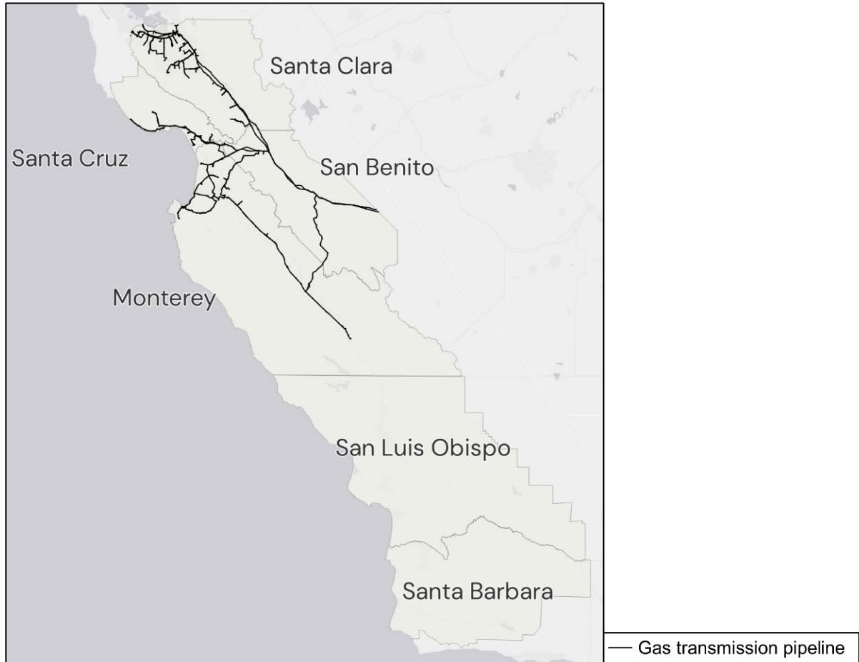
Figure 3.1.2-16. PG&E gas transmission pipelines in the Central Coast Region.
