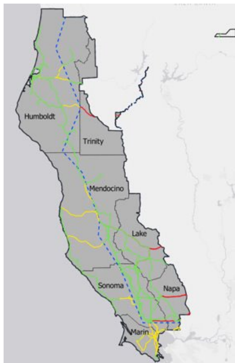
Figure 3.1.1-19. Overhead transmission conductor in the North Coast Region exposed to temperatures at or above the exposure metric for the coastal (yellow) and interior zone (red) in 2050. Conductor in green is not exposed. The boundary between the coastal and interior zones is indicated as a blue dashed line.
